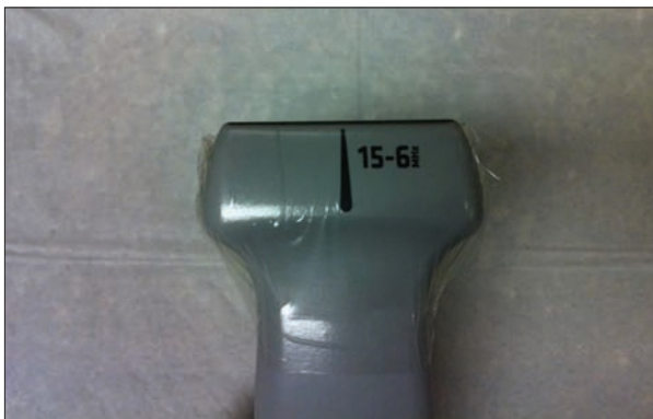
Figure 3: Sterile plastic covering such as 3M™ Tegaderm™ used as an ultrasound probe cover. Reproduced from Macias, M. Ultrasound Leadership Academy: Introduction to Procedural Ultrasound http://www.emcurious.com/blog-1/2014/12/7/ultrasound-leadership-academy-introduction-to-procedural-ultrasound (accessed Sep 6, 2021). Licensed under CC BY 4.0.
